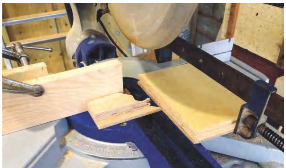
▲ Pic.7 Trimming the feet using the chop saw
